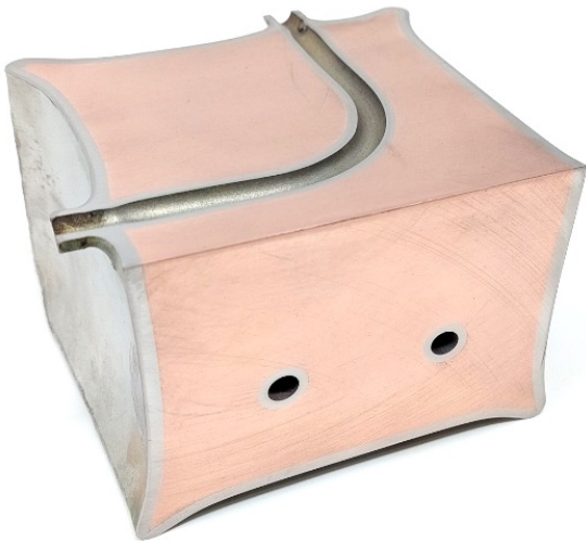
316L cooling channels within a CuCrZr heat sink [cross-sectioned]
