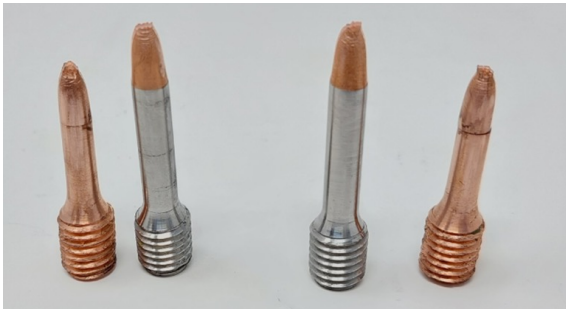
Tensile samples fractured in the gauge section of the CuCrZr indicating good bonding quality of the 316L/CuCrZr interface
